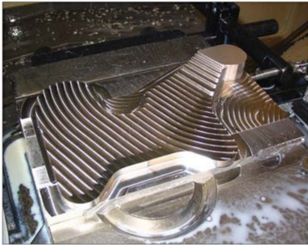
Prior to VoluMill, DMW was using two separate tools to machine this aluminum part with a cycle time of 3 minutes 53 seconds. Using VoluMill, DMW is now able to use one tool and reduce the cycle time to 1 minute 58 seconds.
