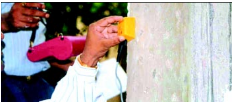
Cover meter or Profometer
